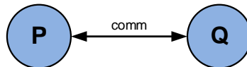
Figure 6.3: Bidirectional synchronisation between processes P and Q using a half-duplex synchronisation event.
