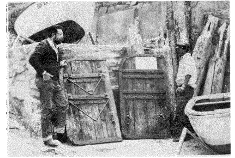
—Foto's: Frik Dreyer Mr G G Clarke (left), curator of the Hermanus Old Harbour Museum, with a pair of otter boards once used by the MARY KATE. The Boards, which serve to keep the mouth of the net open when trawling, were invented by a Scandinavian named Haender, in 1860.
