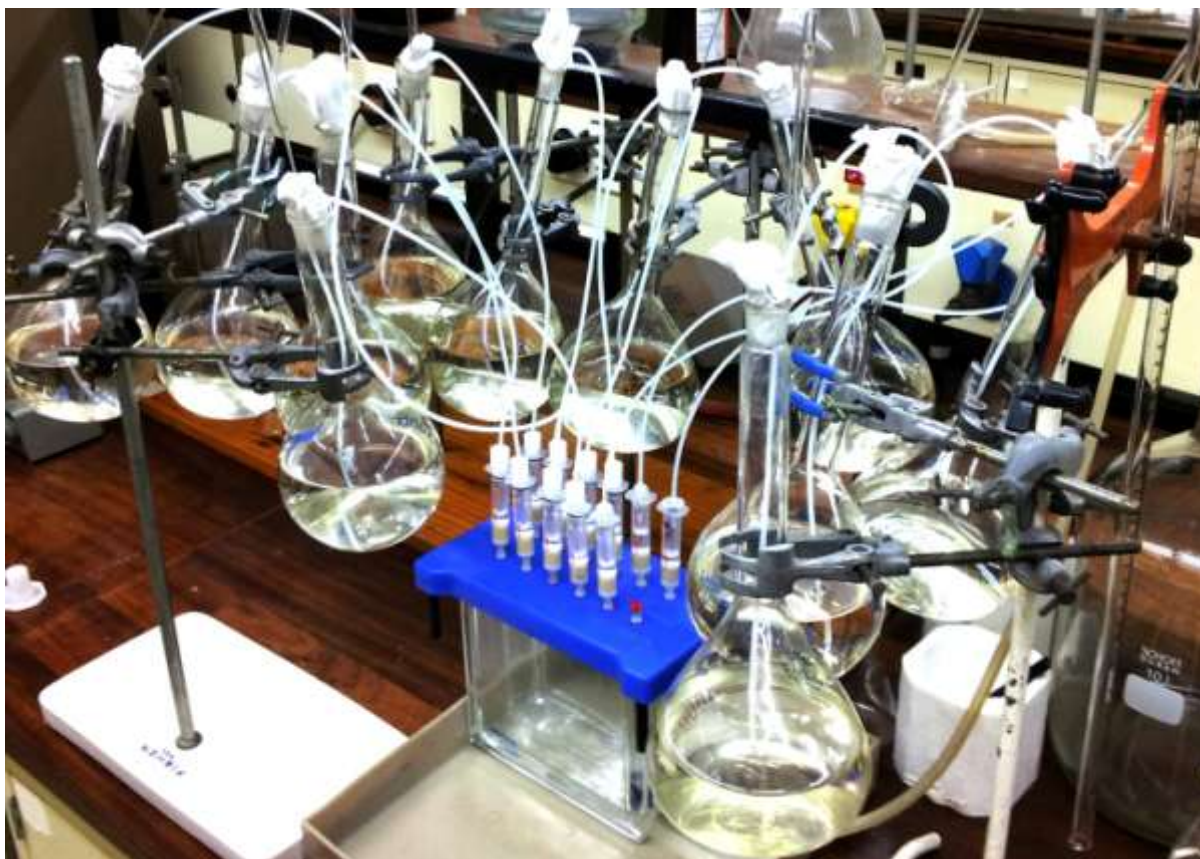
FIGURE 2.3 SPE MANIFOLD SETUP, WITH VOLUMETRIC FLASKS FILLED WITH WASTEWATER SAMPLES.
