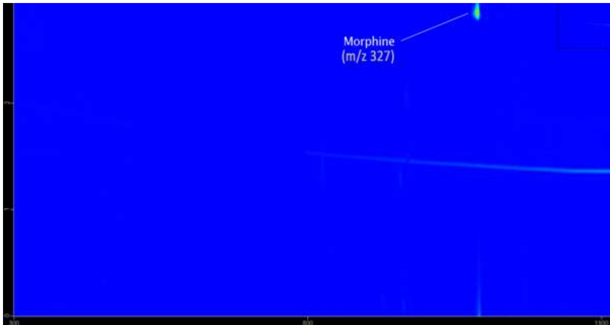
FIGURE 2.7B TWO DIMENSIONAL SELECT ION GCxGC/TOF-MS CHROMATOGRAM OF DERIVATIZED MORPHINE USING (M/Z 327). MS CONDITIONS REPORTED IN SECTION 2.1.2.5.4 MASS SPECTROMETRY.
