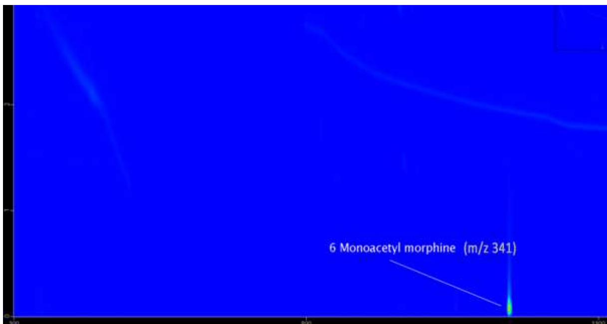
FIGURE 2.8B TWO DIMENSIONAL SELECT ION GCxGC/TOF-MS CHROMATOGRAM OF DERIVATIZED 6 MONOACETYL MORPHINE USING (m/z 341). MS CONDITIONS REPORTED IN SECTION 2.1.2.5.4 MASS SPECTROMETRY.
