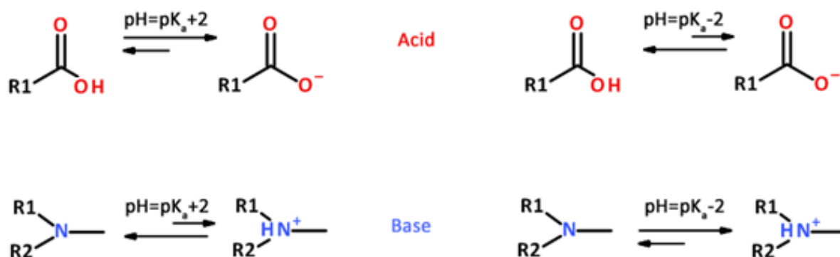
FIGURE 1.14 RELATIONSHIP OF PH TO THE pK_a OF AN ACIDIC OR BASIC FUNCTIONAL GROUP
