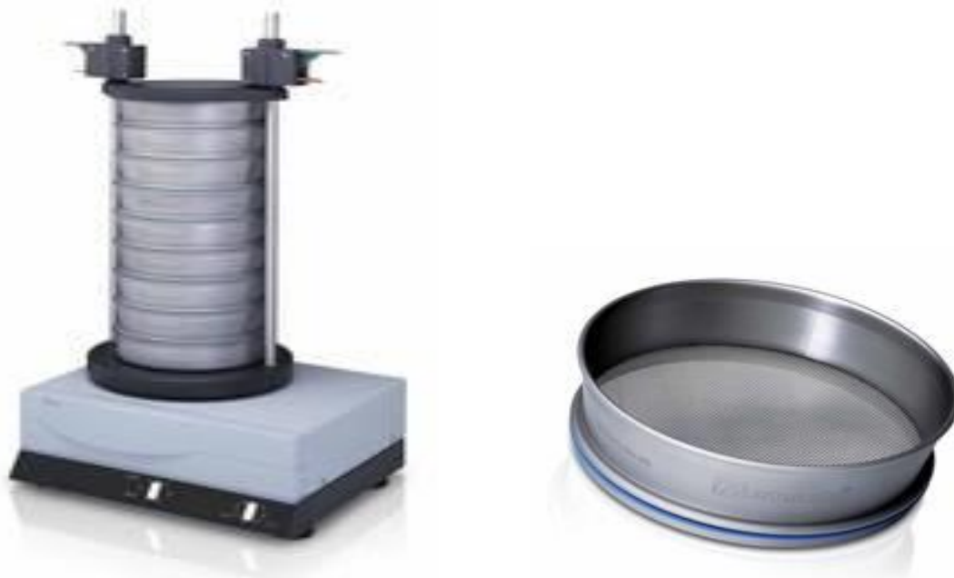
Figure 3.2 Example of Retsch sieve shaker and individual sieve used during this study
