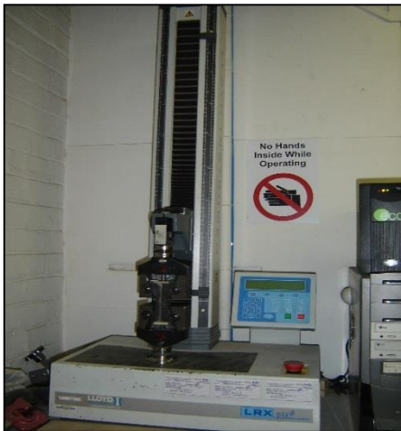
Figure 3.6 LRX Plus Series Lloyd instrument (Civil Laboratory, University of Pretoria)
