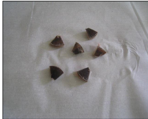
Figure 3.9 Claw disc cut into smaller pieces for milling
