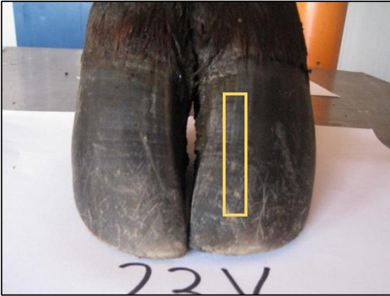
Figure 3.4 Position of rectangular claw sample on dorsal claw wall obtained for tensile strength (TS) testing
