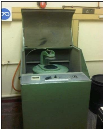
Figure 3.10 Swing mill grinder
