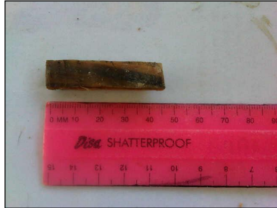
Figure 3.5 Sawn out sample for tensile strength (TS) testing
