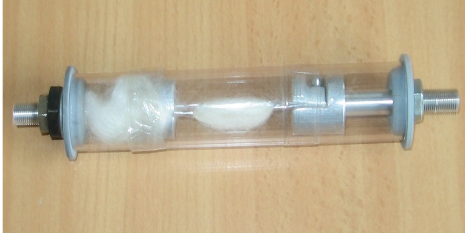
Figure 5.1: SANS sample set-up of the fibres in a quartz tube stretched on both ends for alignment.
