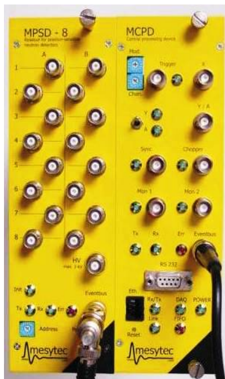
Figure 3.6: Mesytec data acquisition system. Left (MPSD-8): the amplifier module for 8 detectors. Right (MCPD): central processing unit with Ethernet output. Courtesy of http://www.mesytec.com/ (accessed on 23 May 2014).
