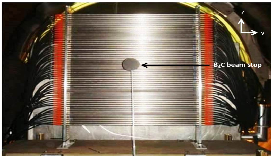
Figure 3.5: 54 ^3\text{He} Position Sensitive Detectors as installed at the Ncsa SANS facility. A \text{B}_4\text{C} beam stop is situated in front of the detectors. The electronics box is housed immediately behind the detectors
