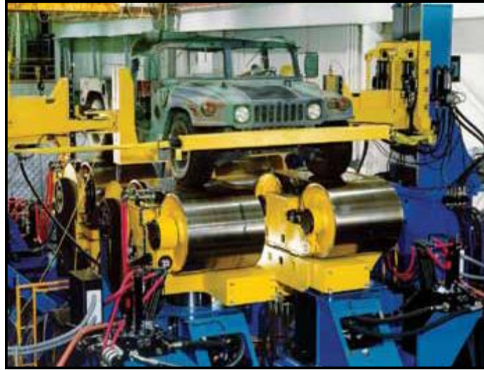
Figure 7: MTS – Flat-Trac Roadway for Dynamic Road Handling testing on large vehicles (Flat-Trac® Tire Test Systems, 2005)
