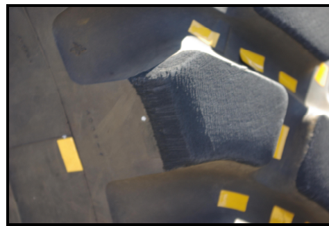
Figure 34: Tyre scrub wear (Michelin tyre)
