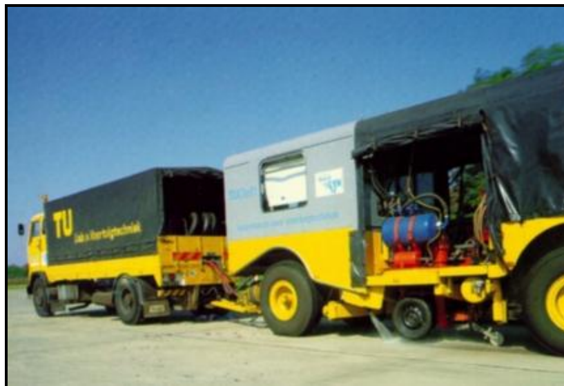
Figure 8: The Delft tyre test trailer (Yunus.hacettepe.edu.tr, (n.d.))
