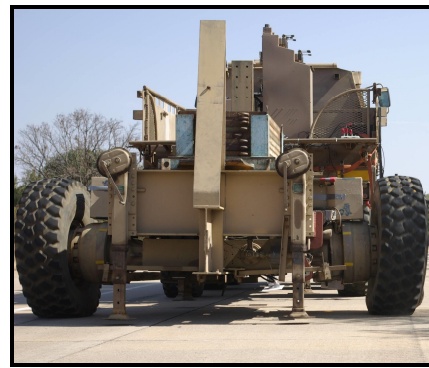
Figure 32: Tow vehicle with Tyre Tester performing slip-angle tests (Michelin tyre)
