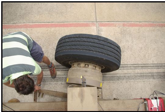
Figure 31: View from top of wheel set at a specific slip-angle (GoodYear tyre)
