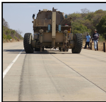
Figure 33: Tyre scrub marks (Michelin tyre)
