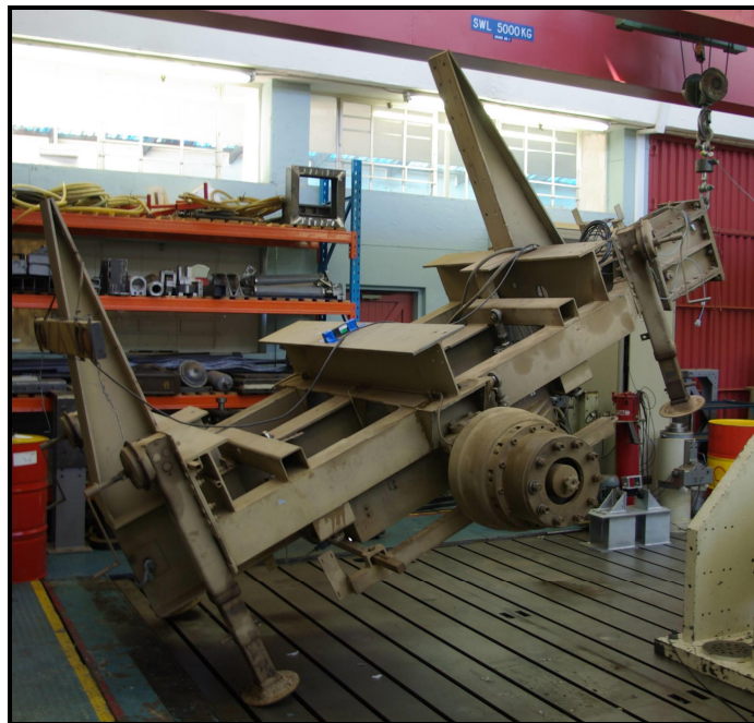
Figure 50: Lift method to determine vertical position of the centre of gravity
