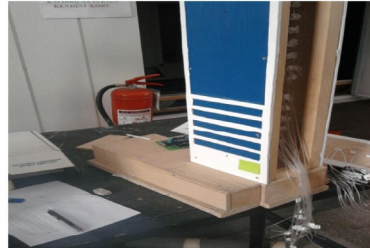
Figure 6 Assembling pressure tubes and cyclones with model
