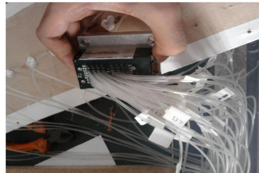
Figure 7 Connection the marked cyclones with transducer
