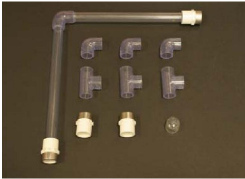
Figure 2: Fittings and 15.29 mm diameter pipes used
