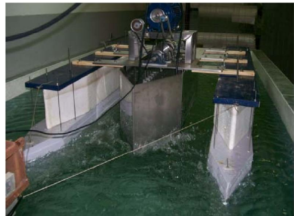
Figure 11. Bollard pull trial under real conditions (fixed pull point).
