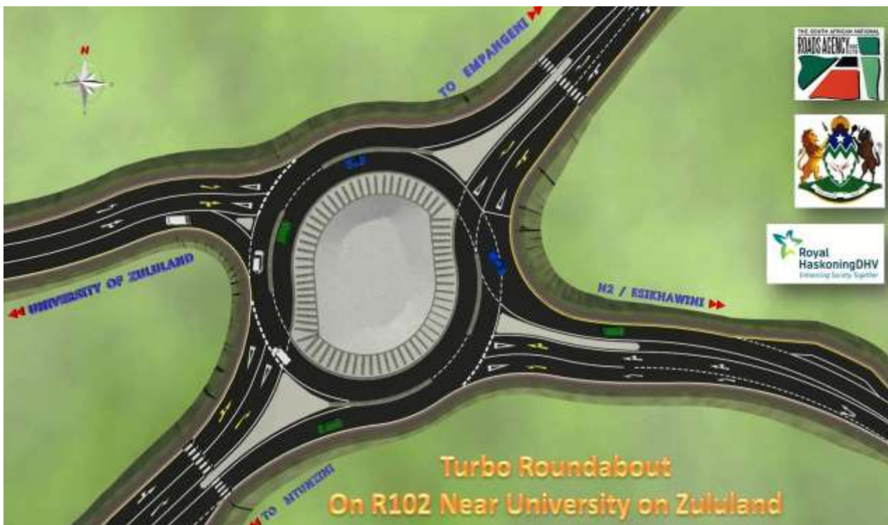
Figure1: Conceptual diagram of the R102 / P535 Turbo Roundabout
