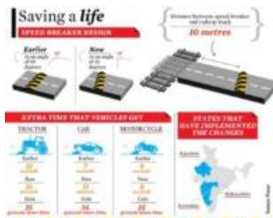
Figure 11(e): Diagonal Speed-Breaker Humps, (N.S. Ramnath and A.K. Mishra, 2012)
