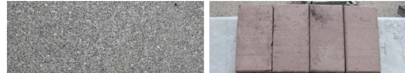
Figure 90- Exposed aggregate concrete & clay brick pavers (Author 2014)
