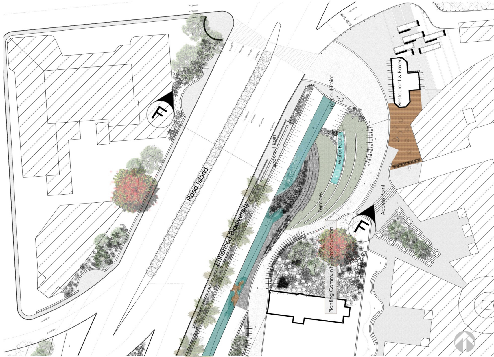
Figure 73 Plan of Scenario 5_River Widening with Terramesh & River Bed modification with Reno Mattress sunken garden (Author 2014)
