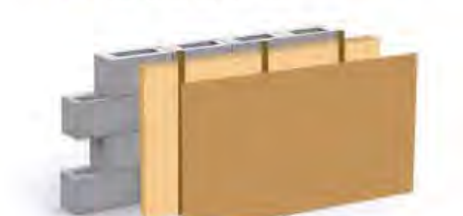
3 single / double skin wall insulation on inside (50mm plastic + 15mm cardboard)
