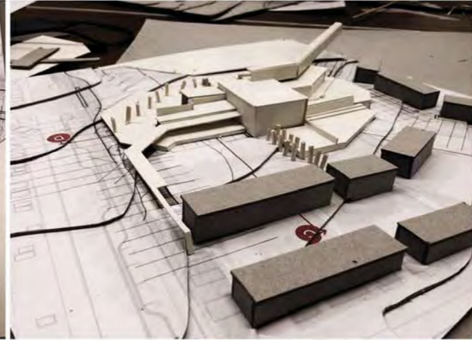
The model is concerned with relative heights and the understanding of its effect on the ground level and surrounding built structures as the movement of water lead to a building being raised out of the drainage route
