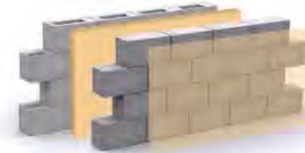
5 cavity wall, 50mm plastic bag insulation in cavity
