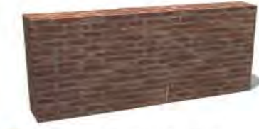
6 commercial cavity brick wall with 20mm EPS
