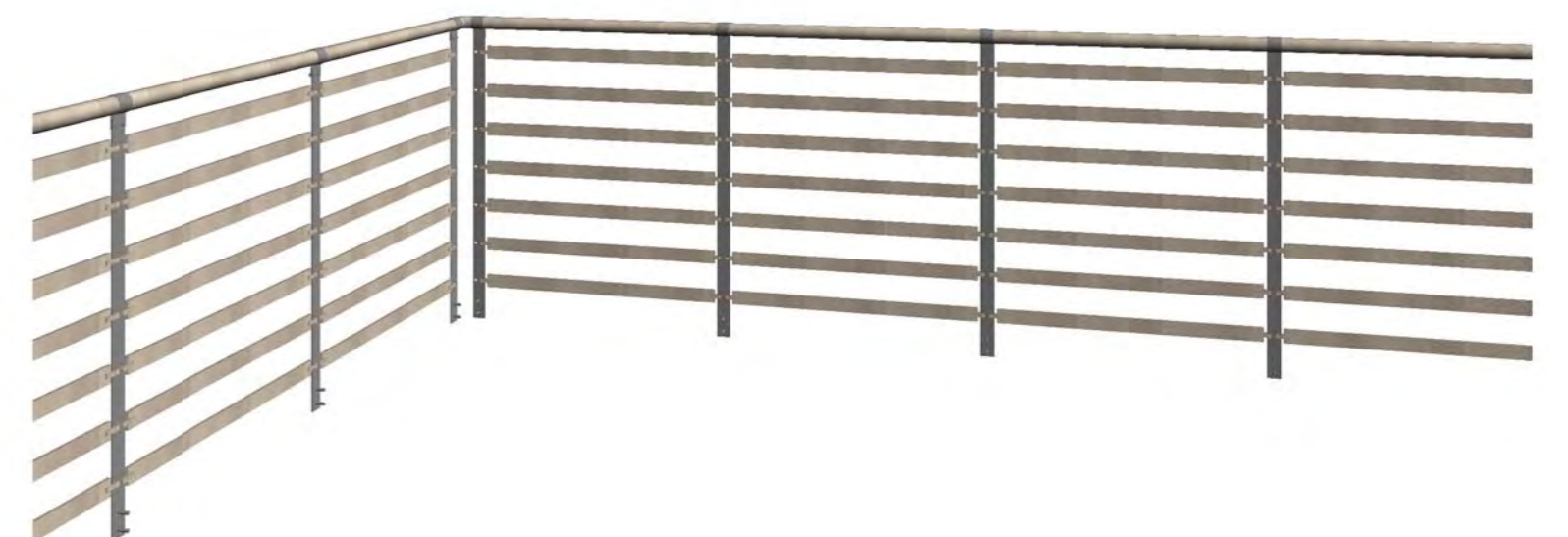
Figure 4.149. BALUSTRADE PERSPECTIVE - INFILL VARIATION -TIMBER SLATS
