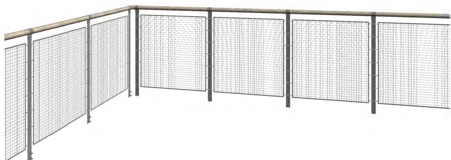
Figure 4.148. BALUSTRADE PERSPECTIVE - WIRE MESH INFILL
