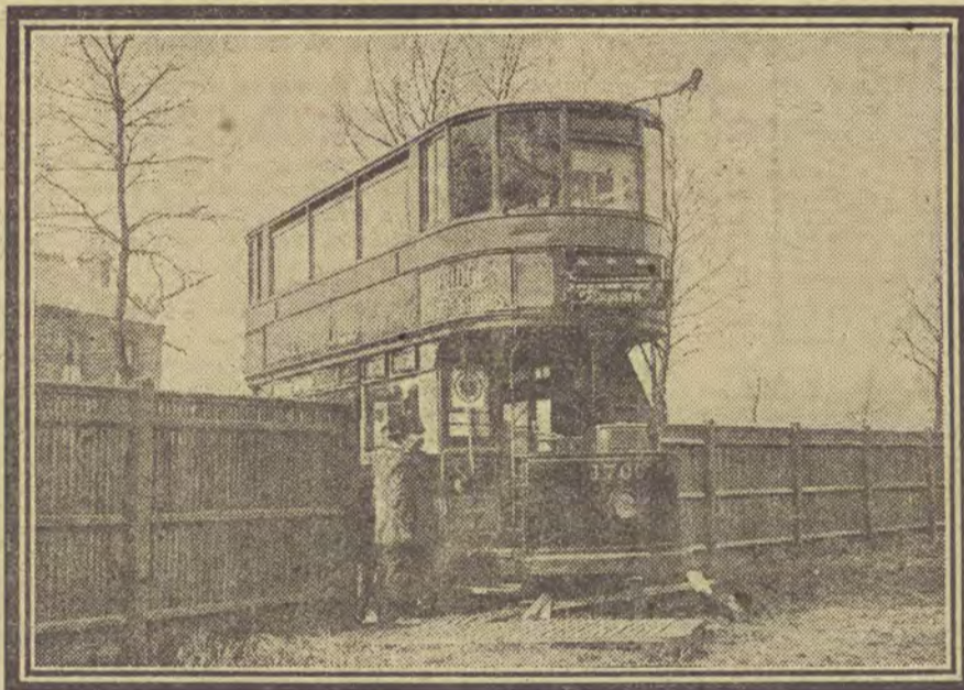
Owing to the brakes failing to act, this tram ran backwards down Dog Kennel Hill, Camberwell, and, jumping the points, crashed through a fence into a field. The passengers had a miraculous escape—not one of them was injured.
