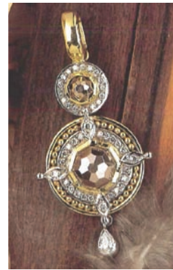
Figure 8—Photograph of Platigems (faceted pink PtAl 2 +Cu) in a jewellery piece (Mintek)
