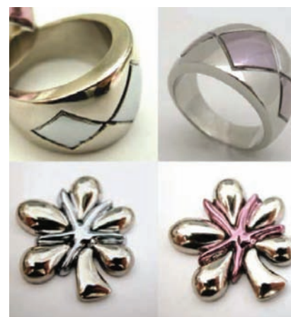
Figure 4—Bi-metal castings of micro-alloyed AuGa 2 blue gold (left) and micro-alloyed AuAl 2 purple gold (right) with 95 wt% palladium (Fischer-Buhner et al. , 2010)
