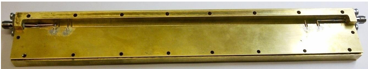
Figure 3.68. Photograph of the inside of the coaxial prototype.
