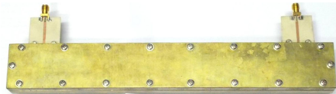
Figure 4.80. Photograph of the exterior of the completed microstrip prototype.
