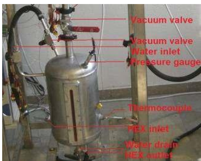
Figure 6 The evaporator and its components
