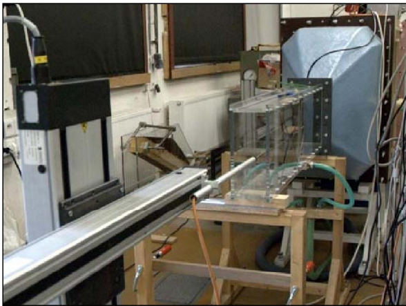
Figure 3 Blow-down test rig with channel and traversing system.
