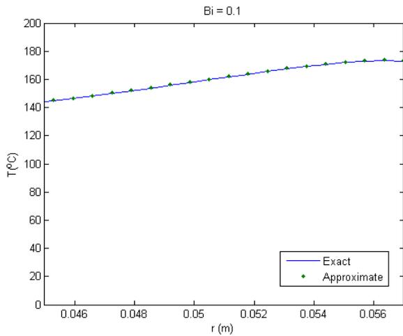
Figure 3: Temperature distribution along the heated surface for  $Bi = 0.1$
