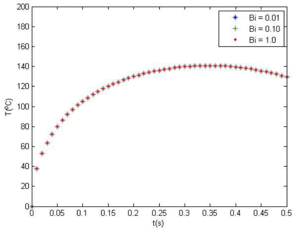
Figure 7: Temperature time history at the mean radius for different Biot numbers
