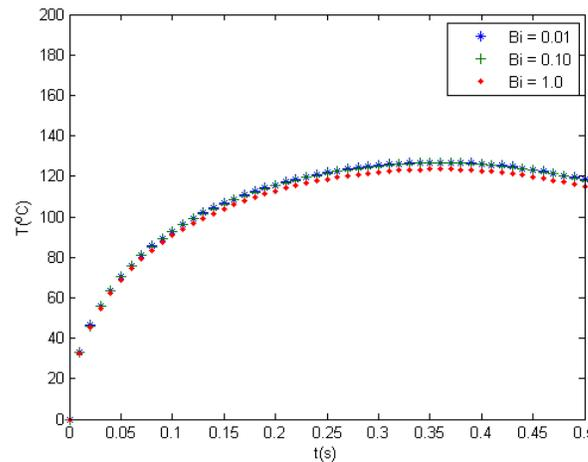
Figure 6: Temperature time history at the inner radius for different Biot numbers
