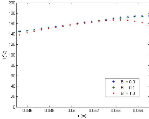
Figure 2: Temperature distribution along the heated surface at the end of the engagement for different Biot numbers.
