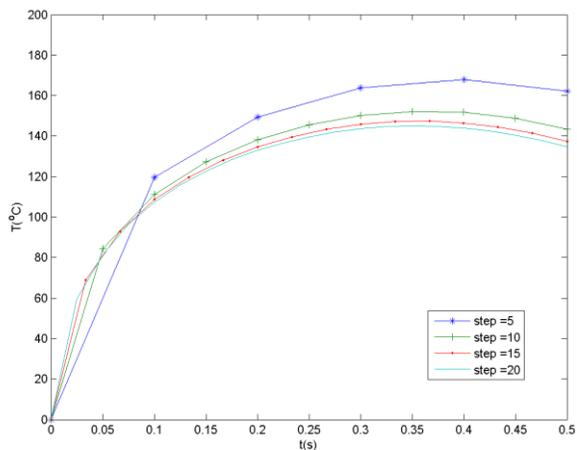
Figure 9: Temperature time history at the mean radius for different number of time steps
