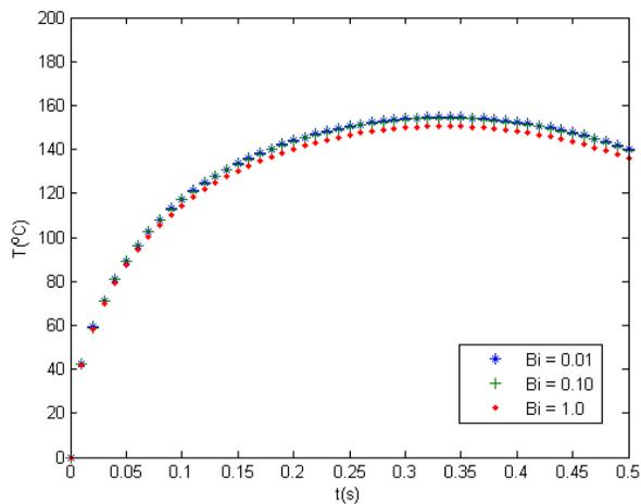
Figure 8: Temperature time history at the outer radius for different Biot numbers
