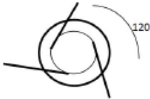
Figure 1 – Rifling Fuel Inlets Increases Mixing
