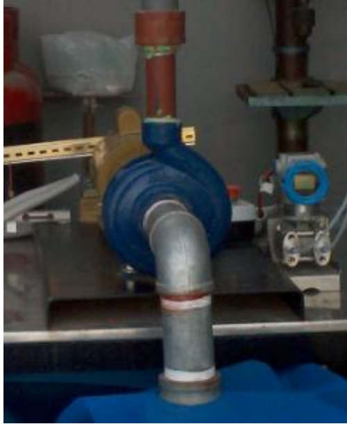
Figure 2 Centrifugal pump working as a turbine.
