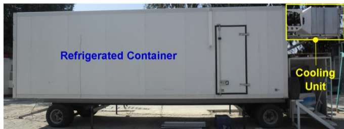
Figure 1 Experimental prototype for refrigerated truck
