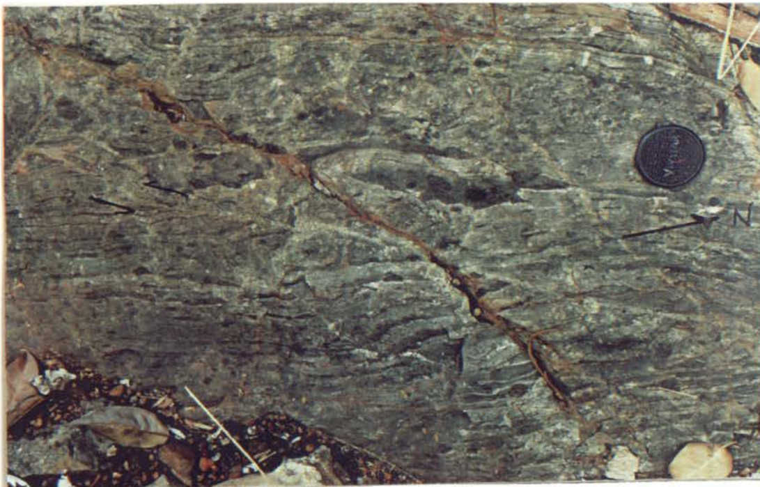
Figure 3.38: Folding and faulting of laminations in Silverton shale at location 24. Sinistral movement has occurred along a fault of strike 025^{\circ} , possibly as a Riedal shear within the Fault zone. Lens cap is 6 cm wide.
