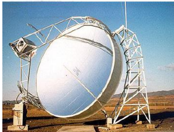
Figure 2.10 Parabolic dish collector with receiver for Stirling engine [36]
