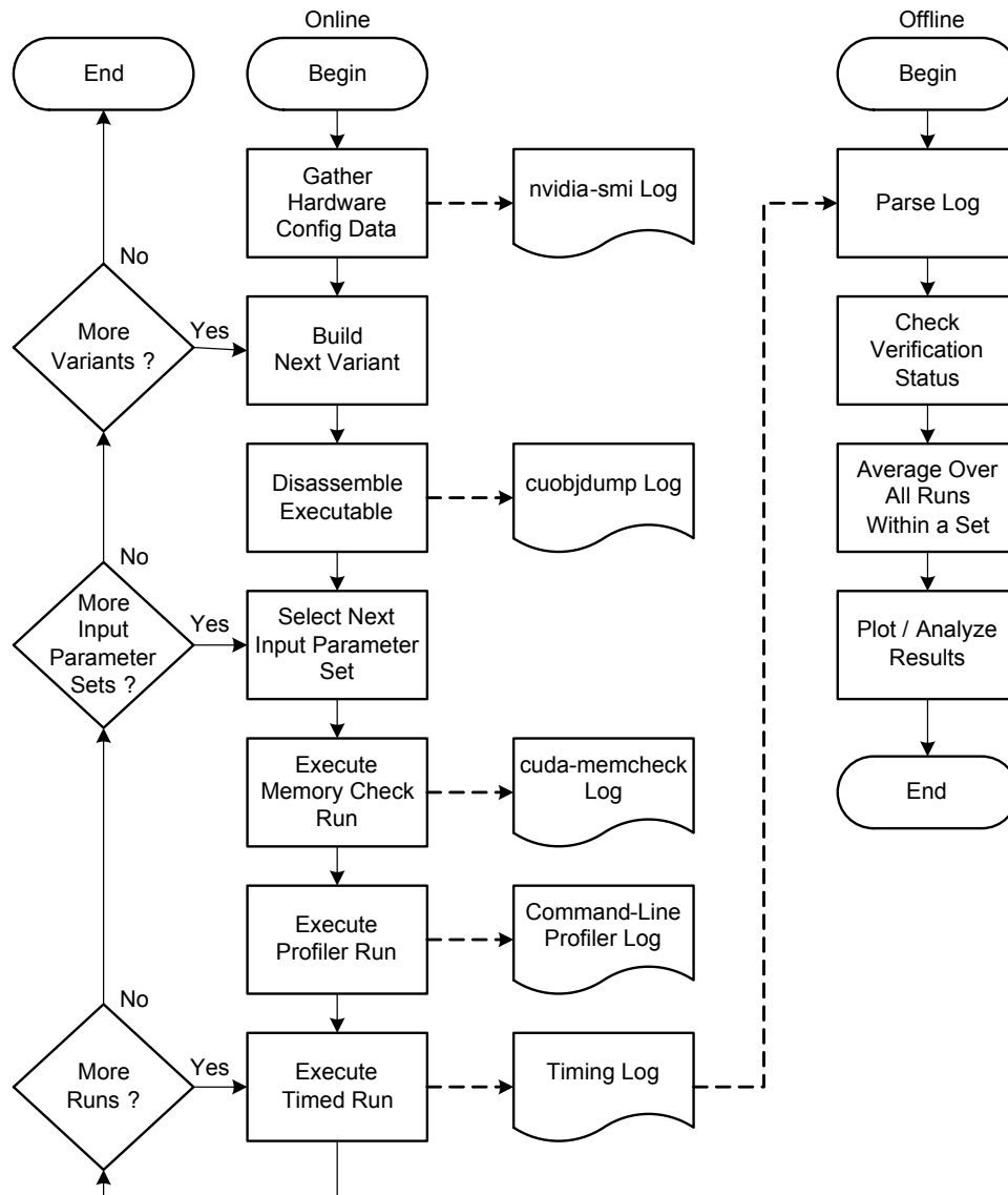
Figure 5.2: Typical GBF benchmarking flow showing outer steps with the online process driven by a BASH script during benchmarking and the offline process driven by a MATLAB script to analyze benchmarking results.
