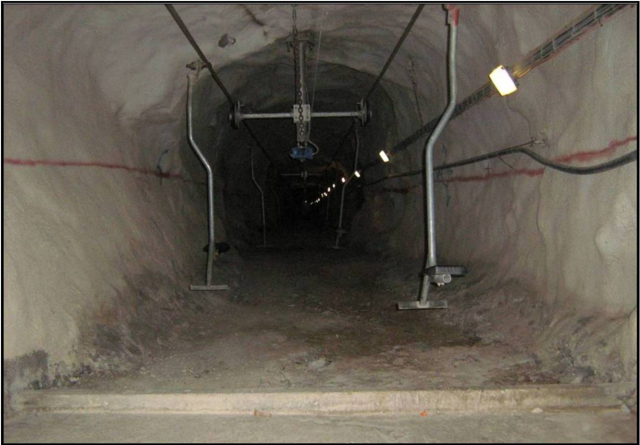
Figure 1.3b: Chairlift installations in the Phase 2 areas of both shafts at BRPM (BRPM, 2008)
