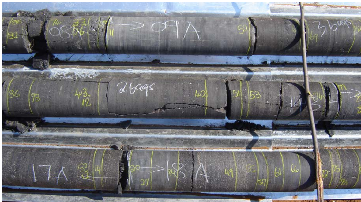
Figure 20 Photograph of typical cores from Grootegeluk Formation coals. The yellow pencil marks are lithology boundaries with associated measured depths below surface. White pencil writing denotes sample numbers and the amount of plastic bags needed to place the material in weighing purposes
