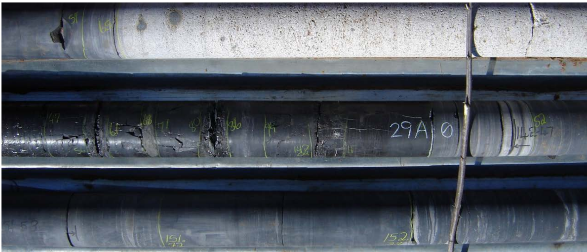
Figure 26 Swartrant coal seams, showing dull coal interbedded with sandstone (coarse, white rock) and mudrock (dark grey laminated rocks). The yellow pencil marks are lithology boundaries with associated measured depths below surface. White pencil writing denotes sample numbers
