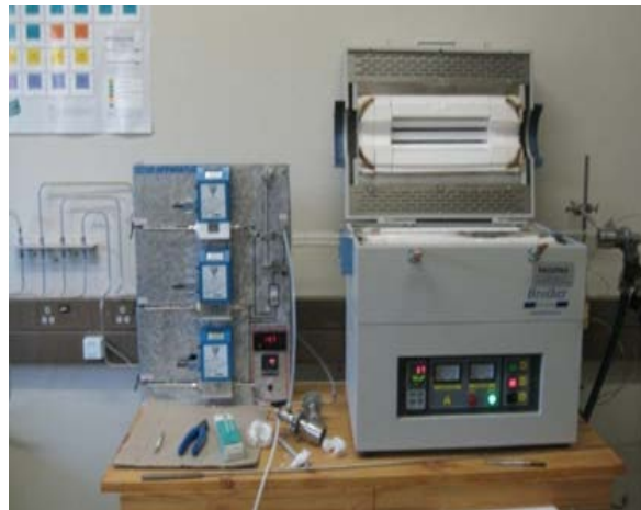
Figure 3.1 Typical thermal chemical vapor deposition system showing different cooling rates of graphene on a nickel substrate.
