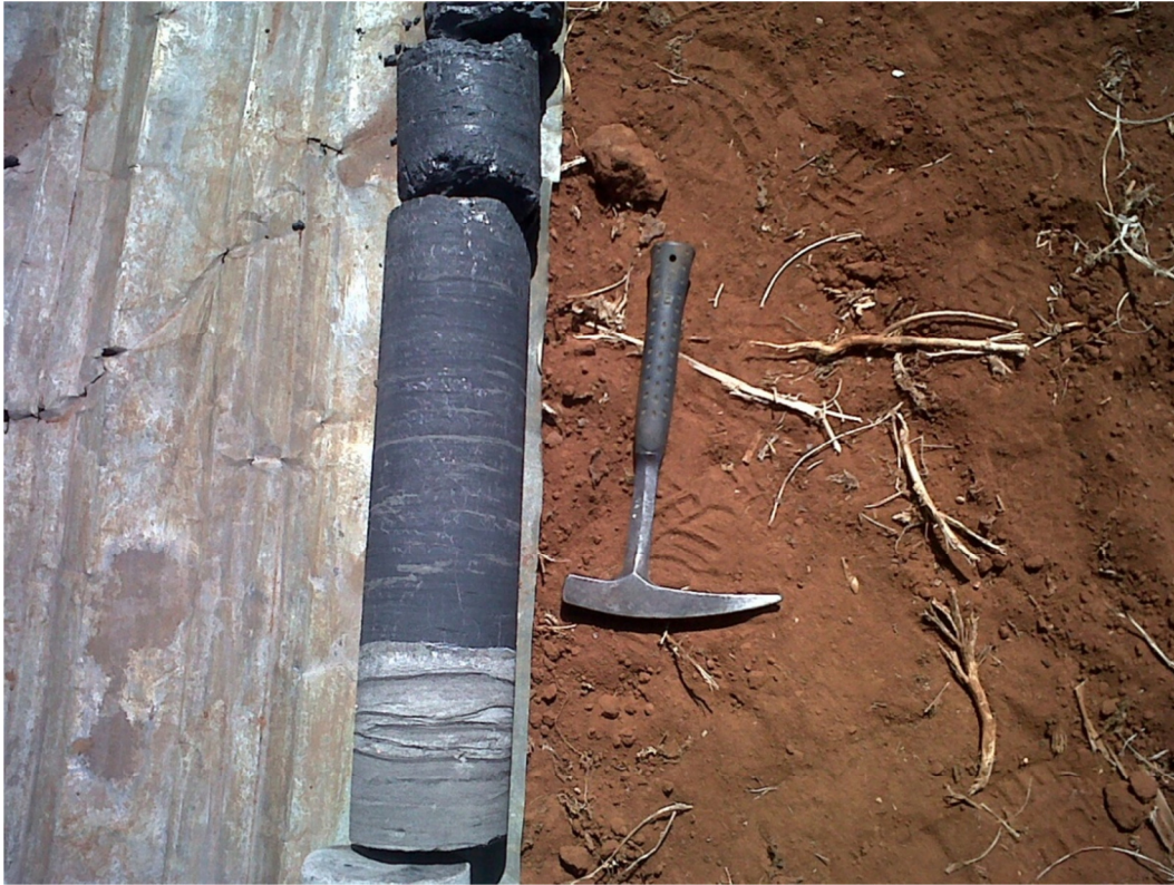
Figure 19. Sharp contact between the lower portion of the top coal seams and the sandstone/siltstone parting separating to and bottom coal.
