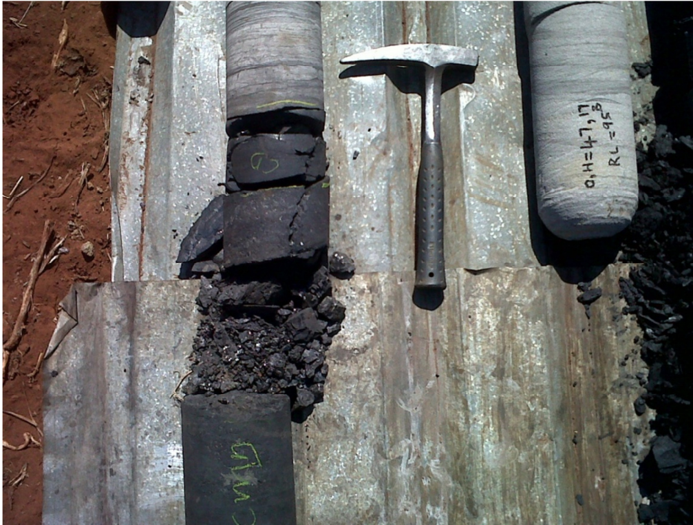
Figure 17. Site drill hole indicating the contact between the sandstone parting and the top coal (40% core loss).
