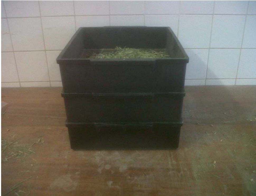
Figure 3.5 The pen state particle size separator with its three trays fitted on top of each other
