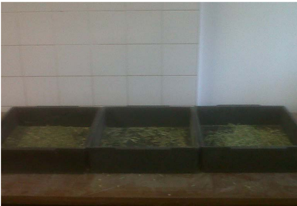
Figure 3.6 The pen state particle size separator with its three trays containing the different size particles
