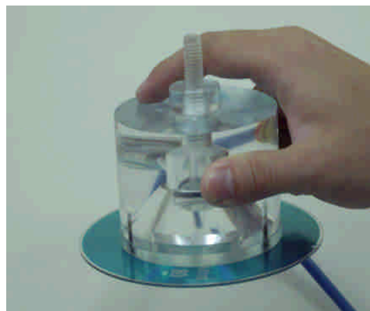
Figure 14 An experimental example showing the developed vacuum pad with a sucked CD-disk
