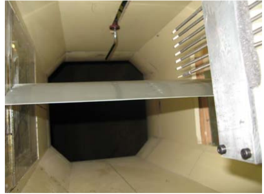
Figure 4 Eppler-361 airfoil in the test section
