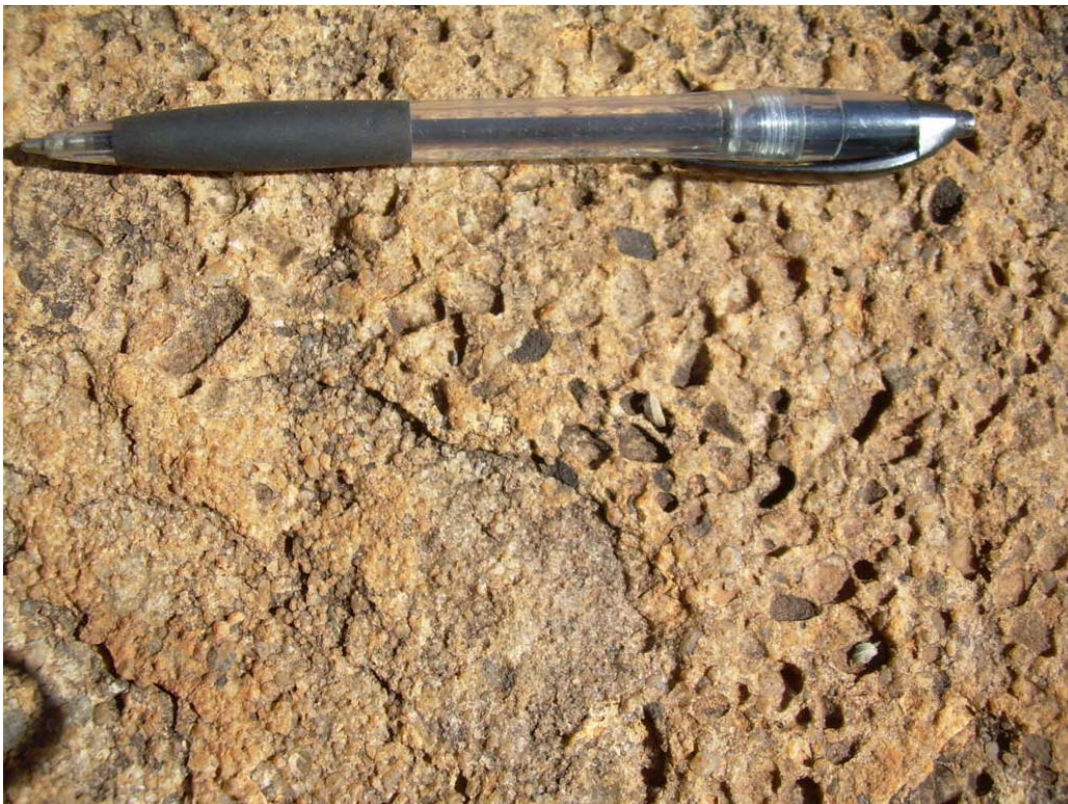
Figure 3.4: Pebbly sandstone from Mothlabeng, western Daspoort basin. Note the bimodal grain sizes.
