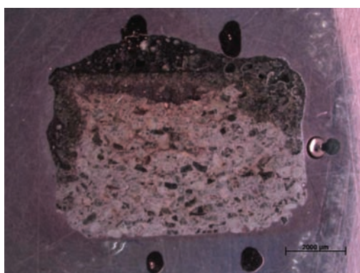
Figure 3—Marra Mamba pellet with darker melt phase penetrating into granular ore phase
