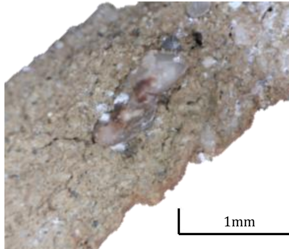
Figure 5.22.2: Distinct quartz grain ( \pm 0.84\text{mm} ) within medium fabric type of vessel 22
