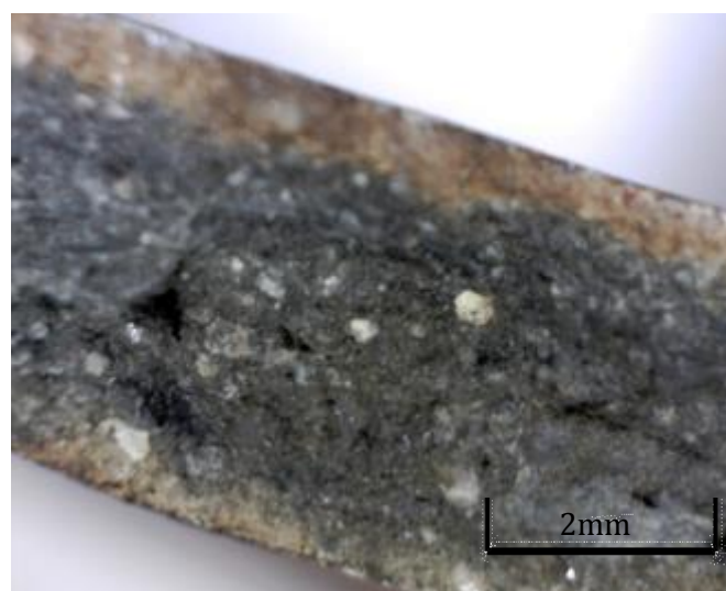
Figure 5.16.3: Fine fabric type of vessel 16 with unoxidized core and sparse amounts of various white inclusions
