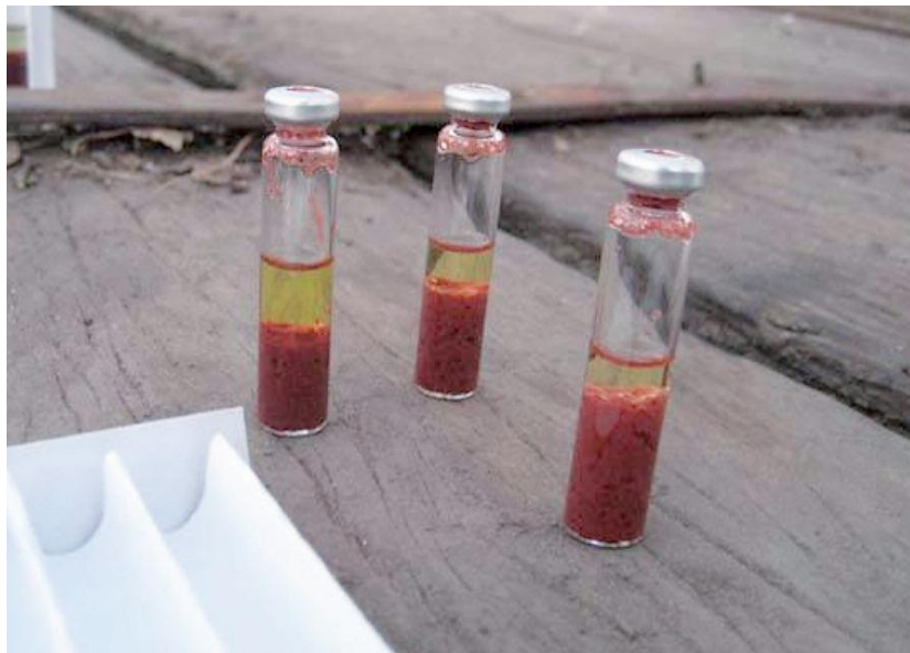
Figure 13 ICheck™ ampoules with sampled blood, absorbing \beta -Carotene into solution for analyses by spectrophotometry
