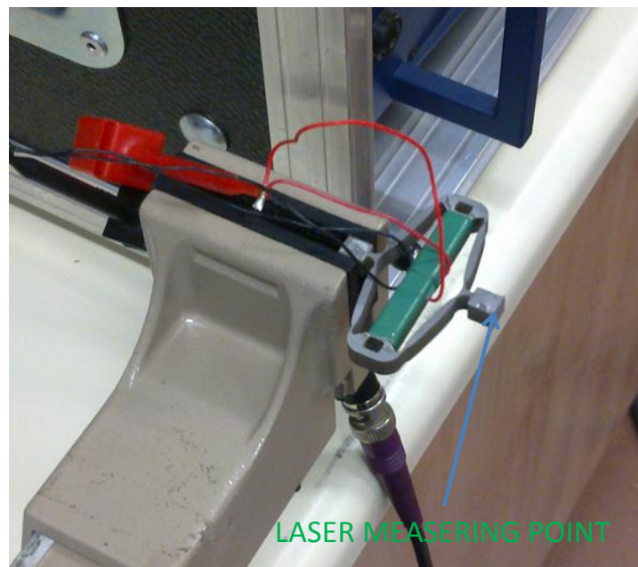
Figure 54: Free displacement measurement set-up
