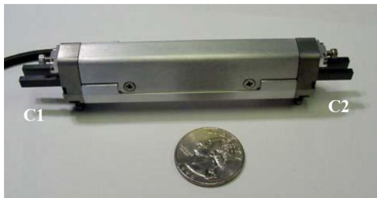
Figure 28: High-power inchworm motor (2005) (Powers et al., 2004)
