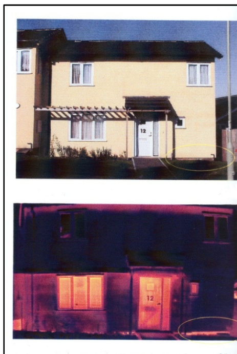
Figure 7 Thermographic image of hemp house constructed at Haverhill research project. Note the difference in colour between the masonry and hemp house (Allin, 2012)
