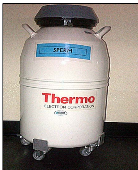
Figure 13: Liquid nitrogen container used for storage of cryopreserved samples (RBL picture library)
