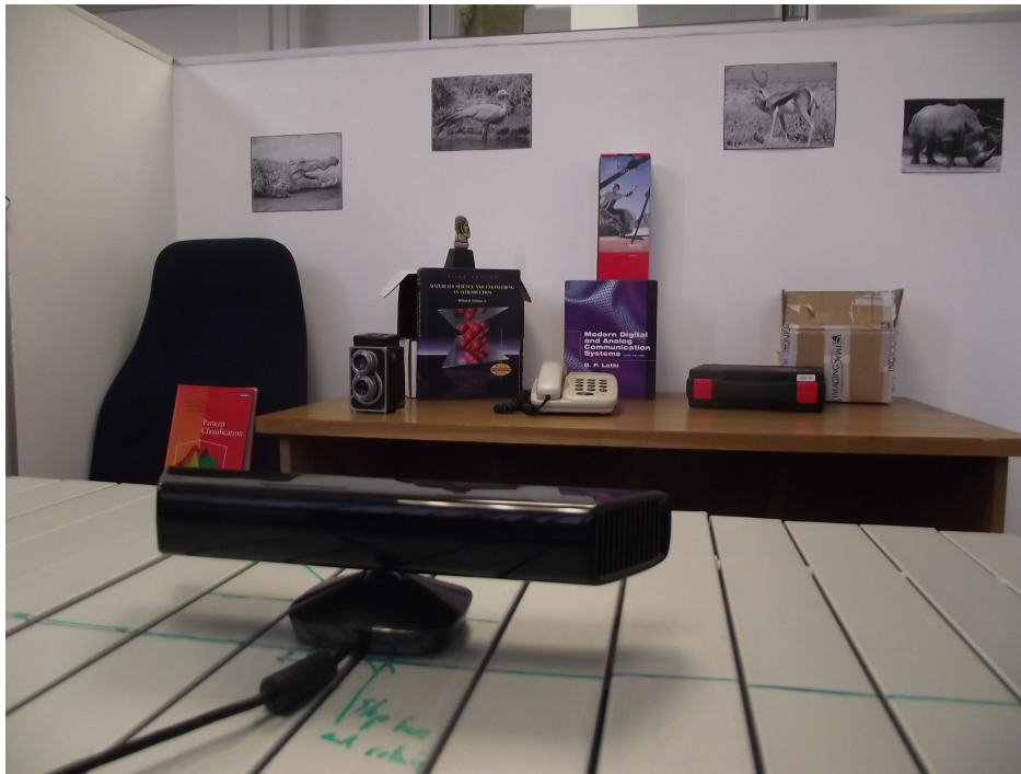
Figure 5.4: Setup for the recording of the Tabletop dataset. Here the Kinect can be seen placed upon the marked path and pointed toward the cluttered desk scene.
