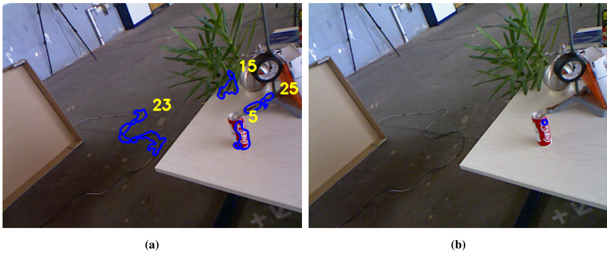
Figure 5.16: Screen captures of the SL and GL SLAM at around time step 250 for the RPY sequence showing how scenes containing low-quality keypoints affected both algorithms.
