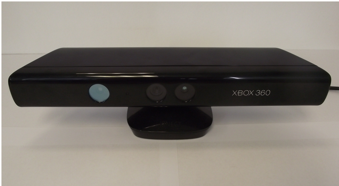
Figure 2.1: Microsoft Kinect. The first circular recess on the left houses the IR laser, the second recess the standard video camera and the third the IR receiver.
