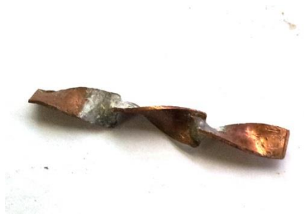
Figure 15 Flow mixer used at the exit of the microchannel to allow for more accurate temperature measurements
