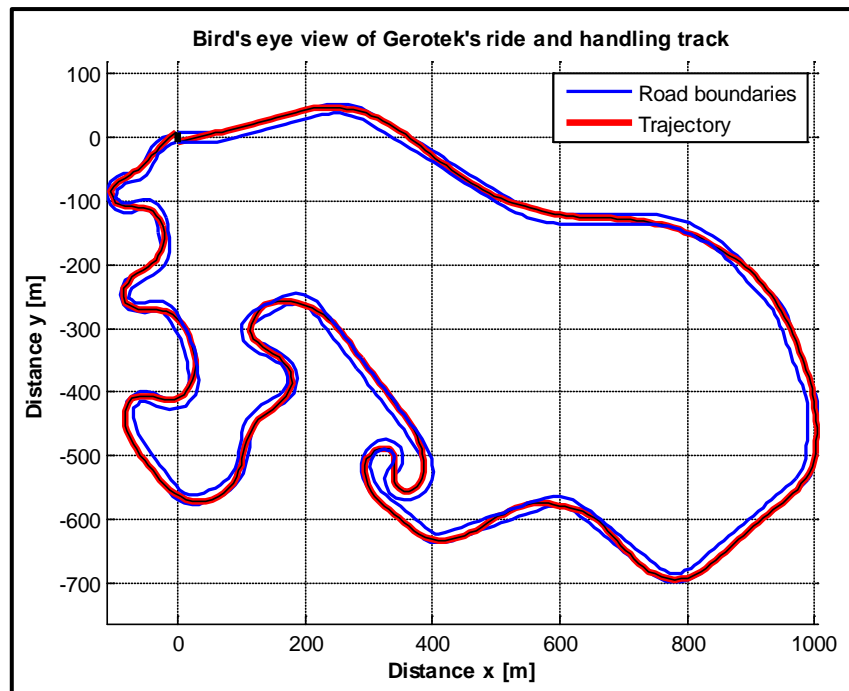
Figure 3.1 – Minimised curvature trajectory of Gerotek's ride and handling track (Gerotek Test Facilities)
