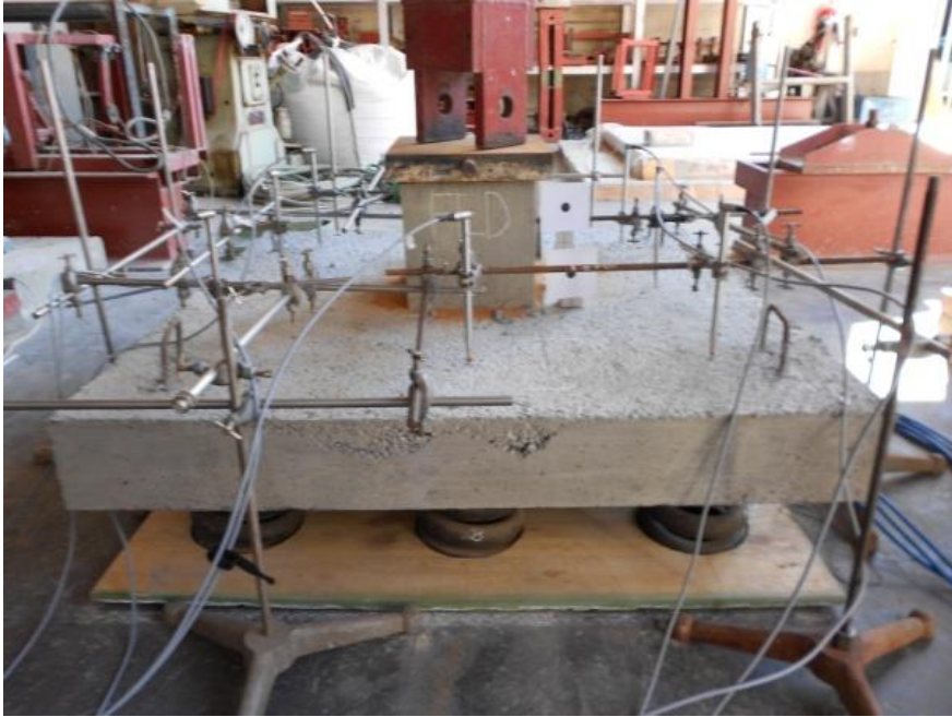
Photo 3-1: LVDT placement on the pad foundation supported on springs (Hossell 2012)
