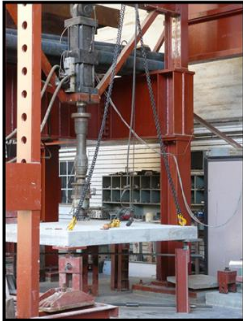
Photo 5-1: Test set-up for simply supported flat slab (Els, 2012)
