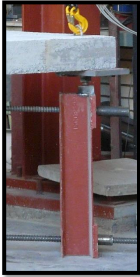
Photo 5-2: Slab supported on ball bearings to ensure rotation is permitted (Els, 2012)
