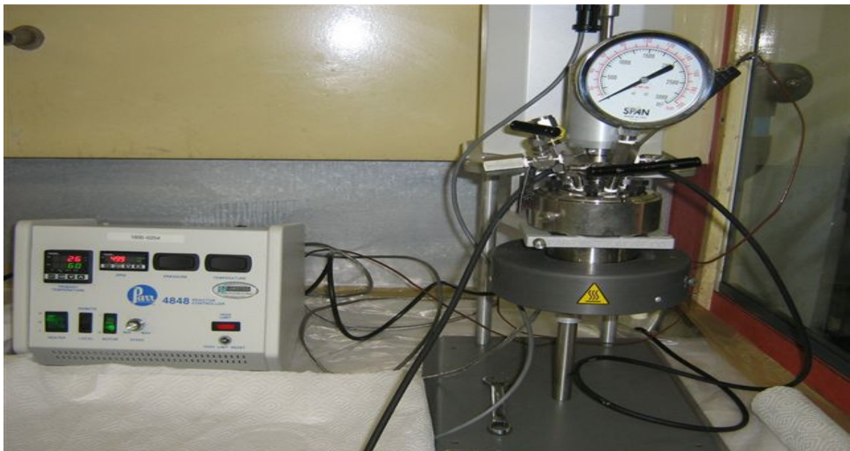
Figure 3-2: Micro Reactor, Moveable Head and a 4848 Reactor Controller
