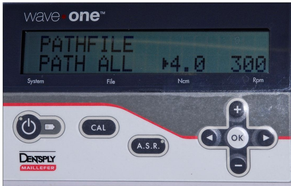
Figure 3.8: The WaveOne Endodontic Motor (Dentsply/Maillefer) set to 300 rpm and a torque of 4 Ncm
