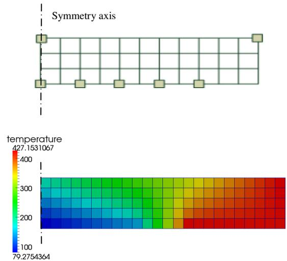
**Figure 3** Domain discretization used for interpolation and resulting temperature map. Please note that only the right side of the plate is represented here.
