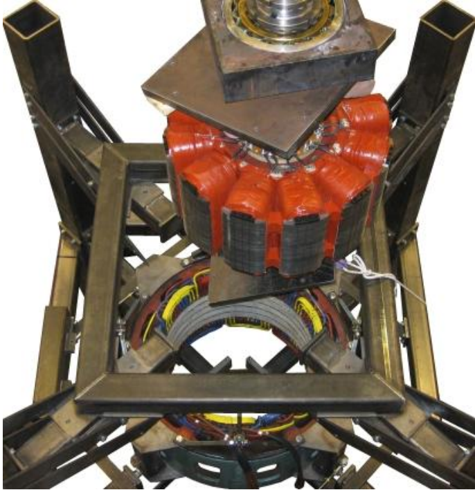
Figure 1: The generator rig used in the experimental measurements, with its main components
