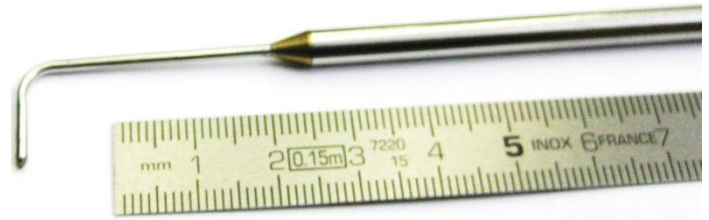
Figure 6: The 5-hole probe used in the measurements
